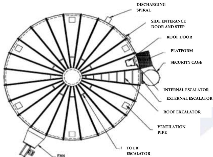
**Note: In conical based silos, there might no be side entrance door, fan and discharging spiral**
