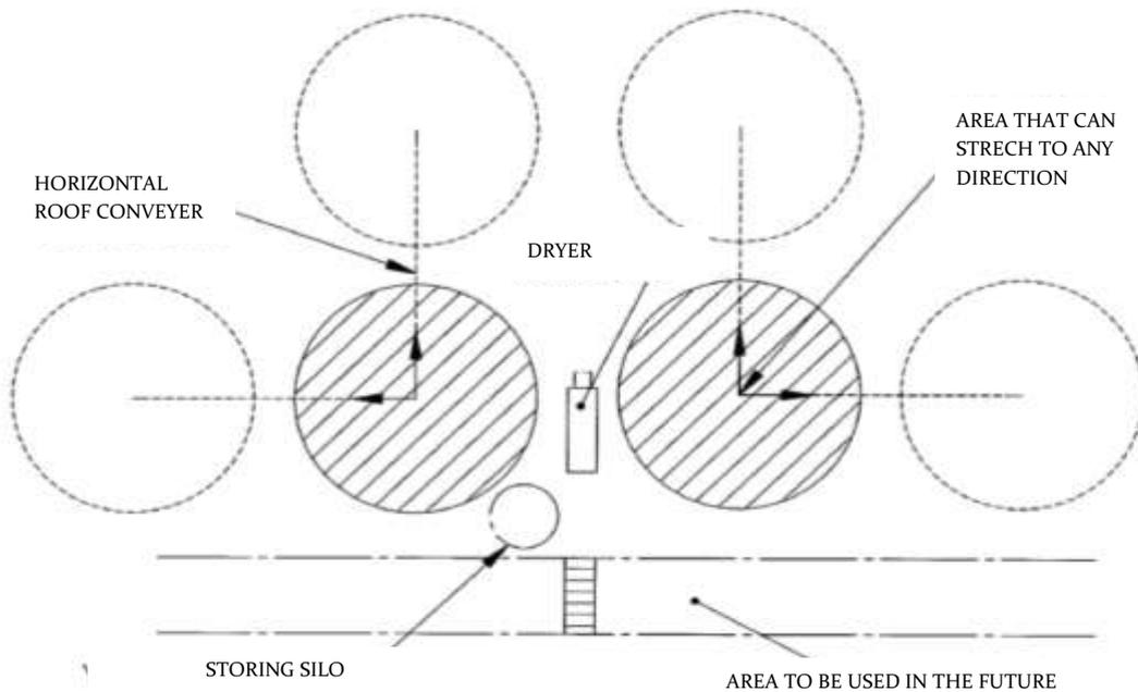
While choosing an area for grain storing and carrying facility or project enlargement, there should be a secure distance to electricity and gas sources and electricity power sources. In American Standards Institute ANSI C7 1997, there is security advice for grain silos. The diagram below indicates the suggested distances between electric cables and grain storing silos and carrying equipment surrounding them.
