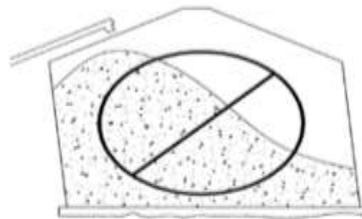
Out-of-center filling may cause turnover or bending and stiffener bendings. Also it may cause turnover momentum in shell plates.
